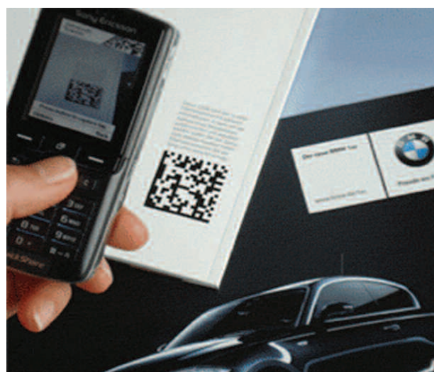
Fig. 11: Mobile devices and iPhones can be directed to URLs using 2D barcodes displayed at the POS. Source: Kemick (2010).
